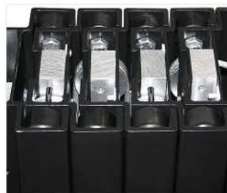
Cable resend system with steel pulleys.
