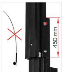
More mast overlap. Prevent fishing rod effect.
