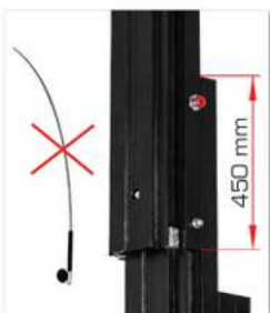
More mast overlap. Prevent fishing rod effect.
