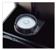
The tower is provided with a **spirit level** to allow it to be vertically
