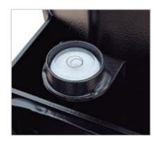
It is provided with a spirit level, for a proper vertical adjustment of the telescopic masts and levelling of the tower.
